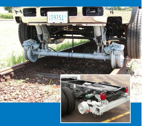
The Harsco Rail MD1920 HY-RAIL® guide wheel equipment is used to adapt medium-duty chassis cab trucks, meeting Harsco Rail's recommended vehicle specifications, for railway applications requiring travel on the highway and on the rail. Featuring hydraulic deployment, hydraulic locks, electrical track insulation, and mechanical safety pins, the MD1920 has a rugged, compact design that continuously provides the durability needed on the track.
