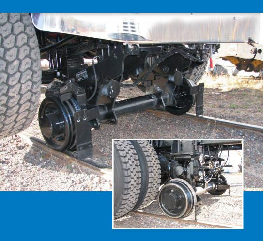
Harsco Rail's HD4141 HY-RAIL® guide wheel equipment is used to adapt heavy-duty, chassis cab trucks, meeting Harsco Rail's recommended vehicle specifications for highway and railway applications. Featuring hydraulic deployment, hydraulic locks, electrical track insulation, and mechanical safety pins, the HD4141 has a rugged, compact design that continuously provides the durability needed on the track.
